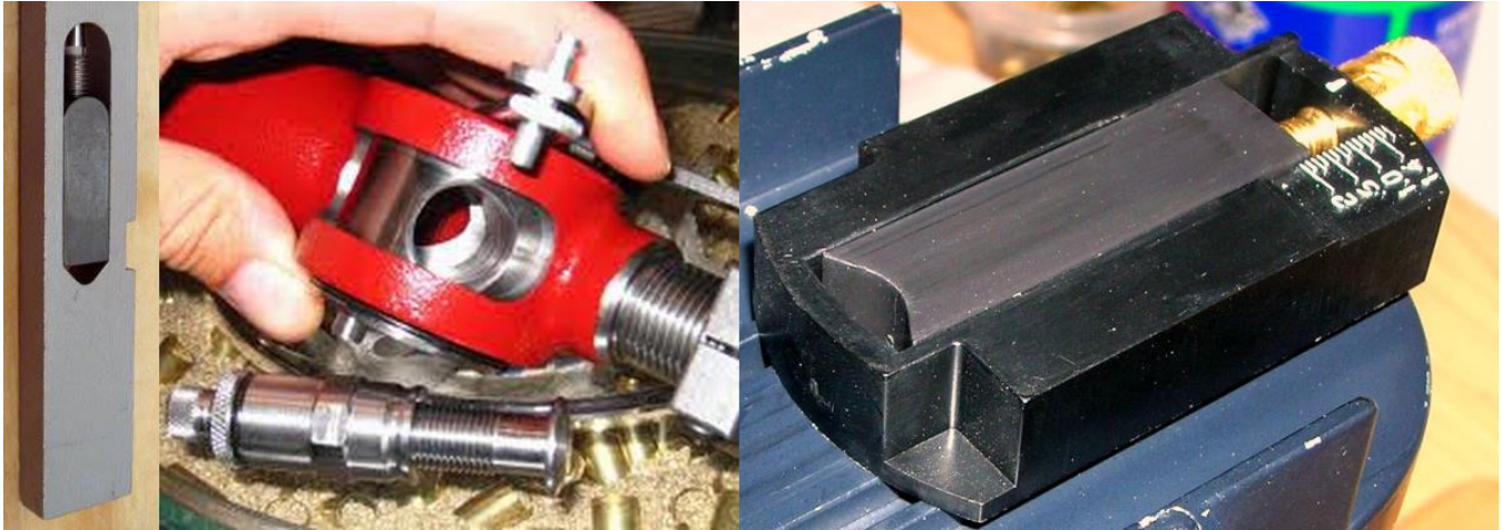
Figure 4 - 650 charge bar, LNL rotor / rifle insert (not micrometer), LM Adjustable Charge Bar
